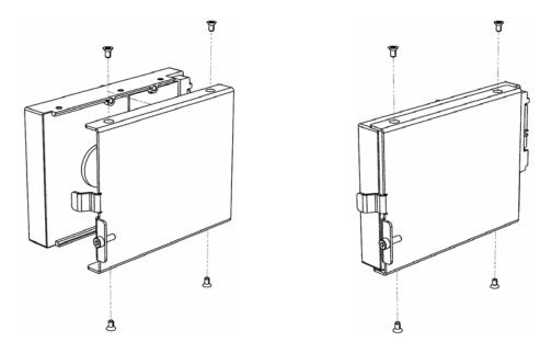
**5** Insert the Hard Drives into the empty hard drive bay and tighten the screws using the 3mm Hex Tool **Note:** Each Hard Drive will only fit in one orientation.
