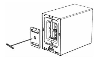
7 Install the Front Cover to finish the installation and protect the drives from fire. Keep the hex tool nearby for future use.
