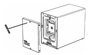
2 Remove Waterproof Drive Cover using the 3mm Hex Tool.
