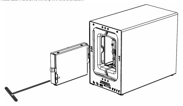
Note: If Drive replacement is required notice that Drive #2 is on the left and Drive #1 is on the right.
