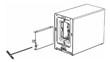
4 Install a compatible Hard Drive into the each Drive Tray using (4x) Drive Screws and a Phillips screwdriver. (Please visit http://iosafe.com/support-2baynas for compatible hard drive models.)
