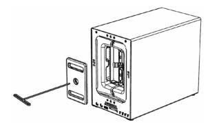
3 Remove both of the Drive Trays using the provided 3mm Hex Tool.
