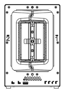
6 Replace the Waterproof Drive Cover and securely tighten using the supplied 3mm Hex Tool.
